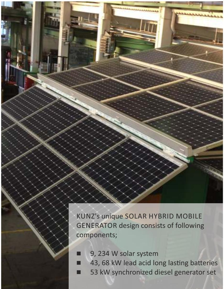
KUNZ's unique SOLAR HYBRID MOBILE GENERATOR design consists of following components;
